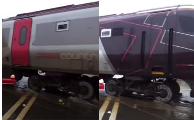
**Figure A5.4 Class 220 passing through a flooded crossing [A5.7]**
