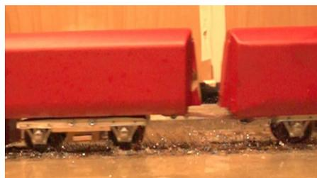
**Figure A4.11 Splashing between Class 43 locomotive and Mark 3 carriage, FFC, 62 mph**
