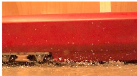
**Figure A4.13 Splashing from the Mark 3 carriage, MWC, 60 mph**
