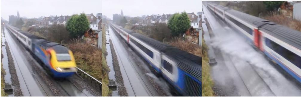
**Figure A5.3 Class 43 passing through flood water at Draycott [A5.6]**
