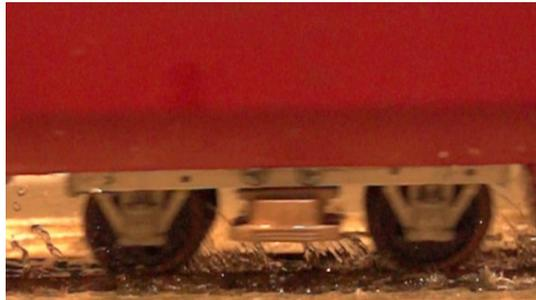
**Figure A4.6 Splashing on Mark 3 carriage front bogie, SFC, 61 mph**
