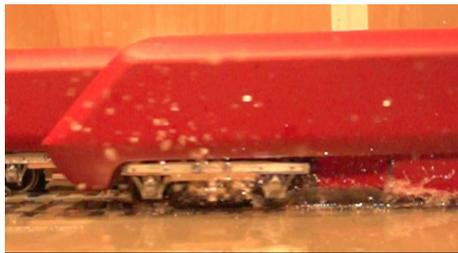
**Figure A4.12 Splashing from the Class 43 locomotive, MWC, 60 mph**
