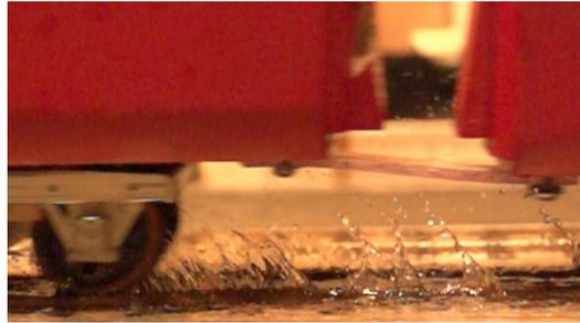
**Figure A4.9 Splashing between Class 43 locomotive and Mark 3 carriage, SFC, 61 mph**
