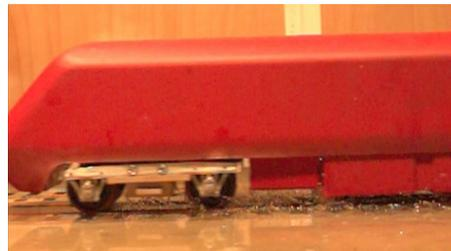
**Figure A4.10 Splashing on Class 43 locomotive, FFC, 62 mph**
