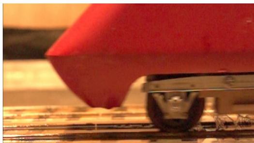
**Figure A4.4 Splashing on Class 43 locomotive front bogie, SFC, 61 mph**
