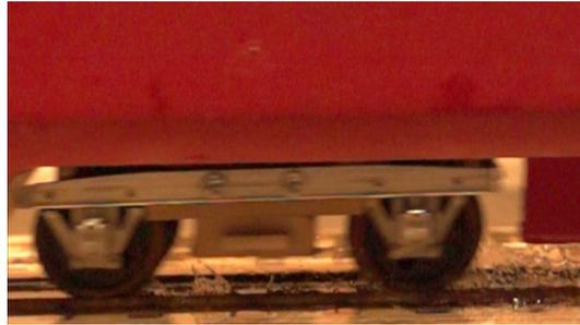
**Figure A4.5 Splashing from front and rear wheels of the Class 43 locomotive front bogie, SFC, 61 mph**
