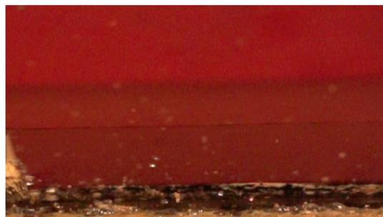
**Figure A4.8 Splashing on Mark 3 carriage underbody, SFC, 61 mph**
